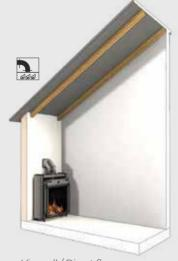
Via wall / Direct flue · direct to the fire with a 90° bend to the exterior
